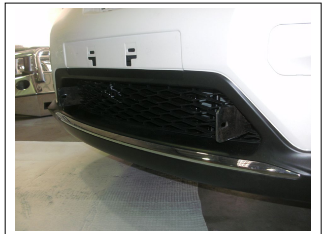
Figure 10: ECB steel mounting bracket with bumper fitted
