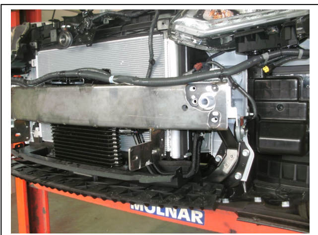
Figure 5: ECB Steel mounting bracket fitted.
